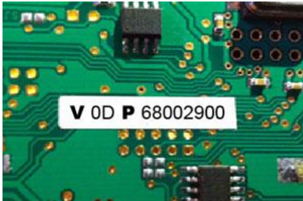
Figure 63: Unique ID on Assembly
