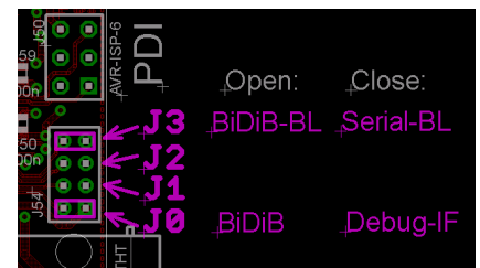
Figure 50: GBM bootloader jumper
