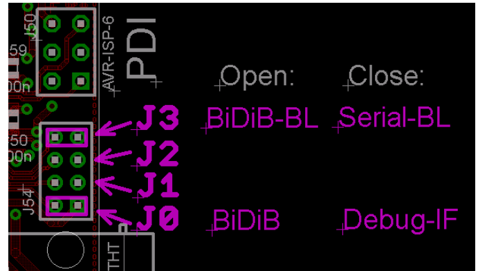
Figure 38: GBMboost bootloader jumper
