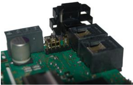
Figure 19: GBMboost v1. 8 heatsink
