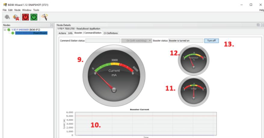
In the booster current diagram (10.) the current (load) of the last seconds to minutes are displayed graphically. With the buttons “Turn on/Turn off” (13.) the ReadyBoost can be switched on or off.
